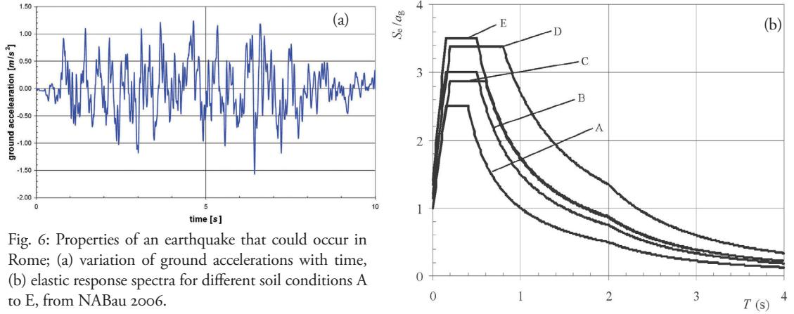
Fig. 6: Properties of an earthquake that could occur in Rome; (a) variation of ground accelerations with time, (b) elastic response spectra for different soil conditions A to E, from NABau 2006.
