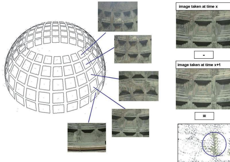
Fig. 9: Monitoring by differential analysis of images taken at different times.
