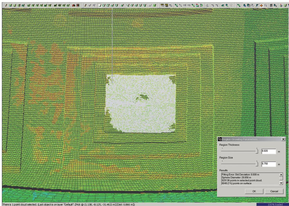
Fig. 9: The internal surface of the *lacunars*, approximated by a sphere (worse).
