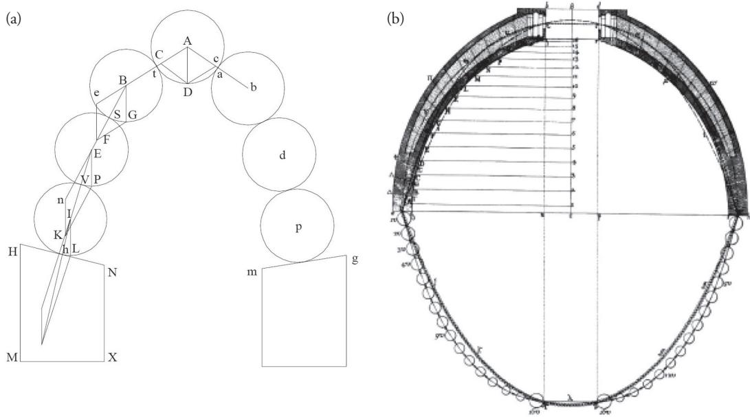
Fig. 3: Construction of the thrust line according to Poleni 1748; (a) represented by spheres, redrafted by Cáncio 1996; (b) represented by a catenary, loaded proportionally to the cupola's weight.
