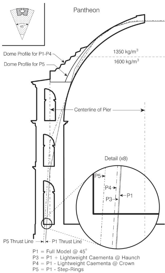
Fig. 10: Pantheon. Results of thrust line analysis.
