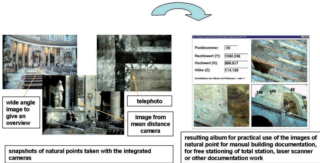
Fig. 5: Left, automatic documentation (from wide-angle to telephoto images) using a video total station; right, album for the practical use of the images of natural point for manual building documentation, for free stationing of total station, laser scanner or other documentation work
