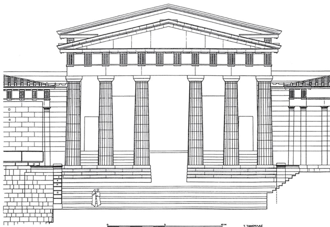
Fig. 14: The Propylaea of the Acropolis, Athens, west elevation (T. Tanoulas, in J. Niels, *The Parthenon from Antiquity to the Present* (Cambridge and New York 2005), fig. 44b).
