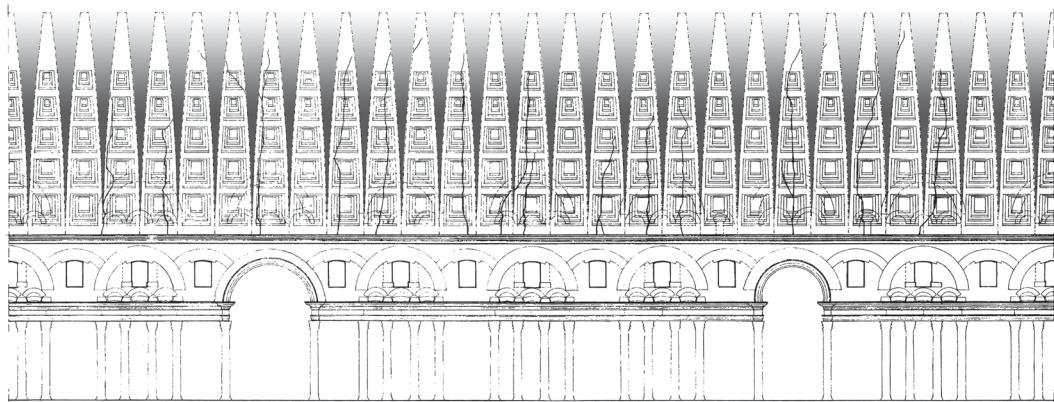
Fig. 4: Orthogonal projection of the interior of the Pantheon showing the principal cracks, after Terenzio (Ippolita D'Ayala Valva, in Wilson Jones 2000, fig. 9.21a).
