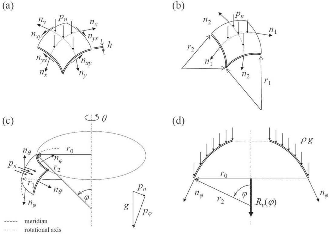
Fig. 1: Membrane theory: (a) out-of-plane loading and membrane forces, (b) principal normal forces and according radii, (c) denominations of shells with rotational symmetry, (d) radial normal forces due to gravity loads above.
