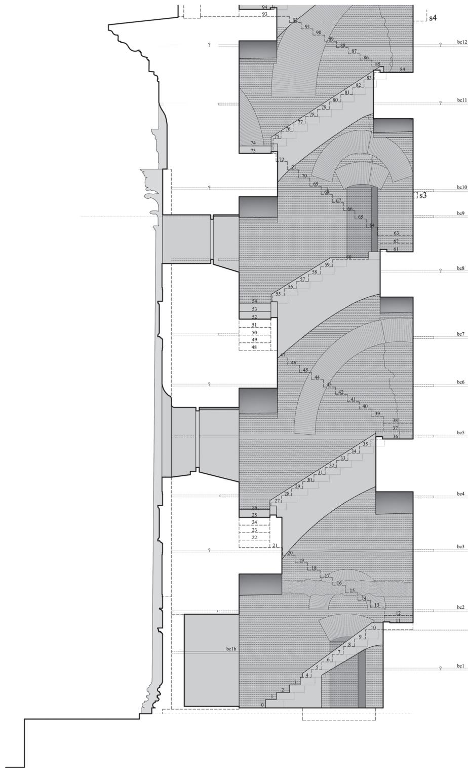
Fig. 9: Detail section/elevation of the lower half of the East Stair, 1 : 100 (author and Robert Grover).
