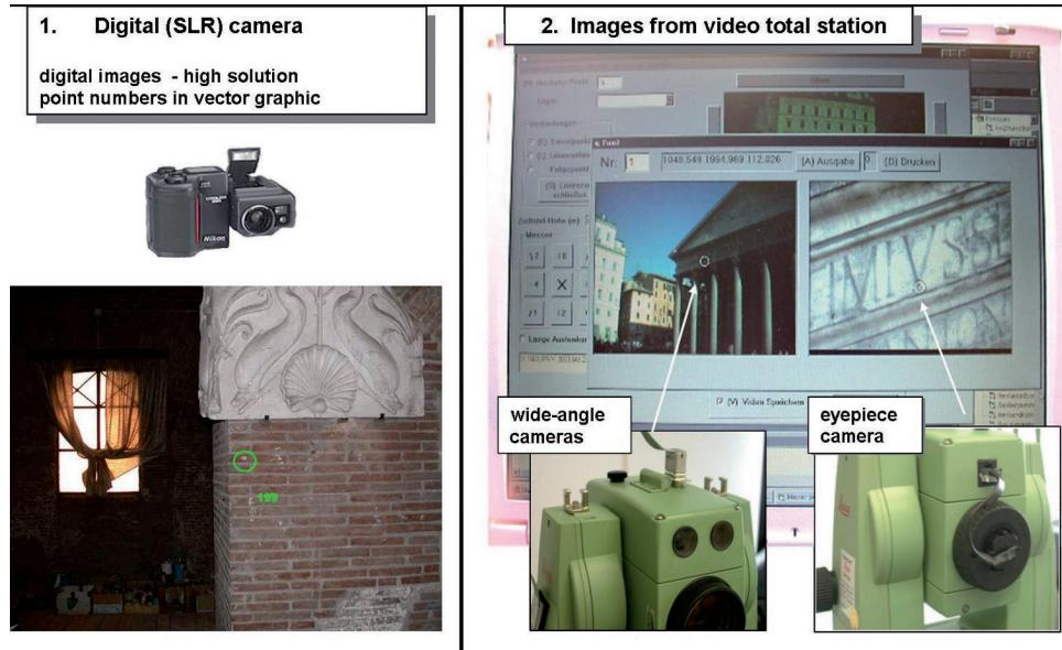
Fig. 4: Alternative ways of documenting natural points: left, with a digital camera; right, using the cameras of the video total station.
