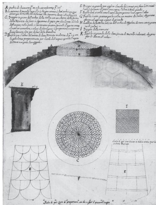
Fig. 6: Glazing of the *oculus* from the reconstruction project under Pope Alexander VII.
