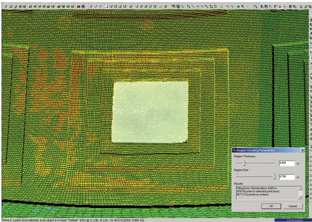
Fig. 8: The internal surface of the lacunars, approximated by a plane (better).
