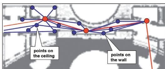
Fig. 1: Object-bound micro-networks replace the traverses (the red lines represent the traverses while the blue lines represent the measurements to natural points on the walls or the ceiling).
