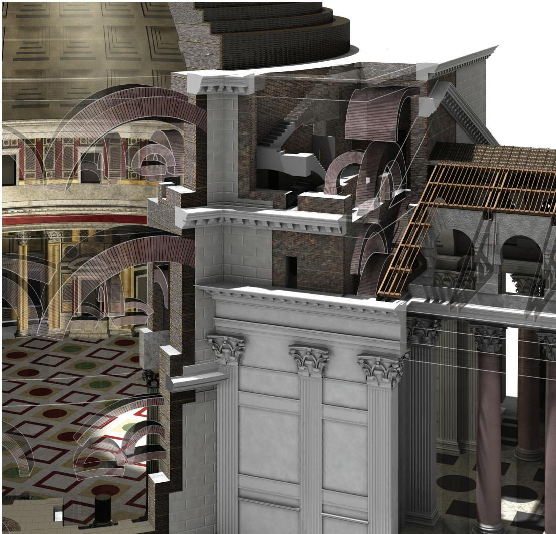
Fig. 10: Cut-away of a 3-dimensional virtual model of the Pantheon (Robert Grover).
