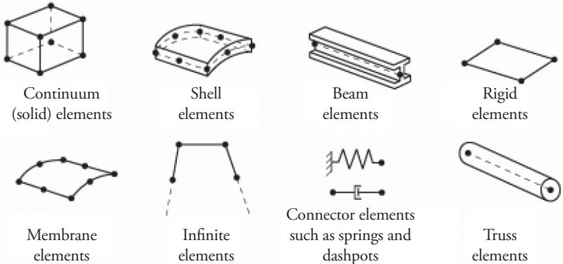
Fig. 5: Commonly used families of finite elements, from ABAQUS 2004.
