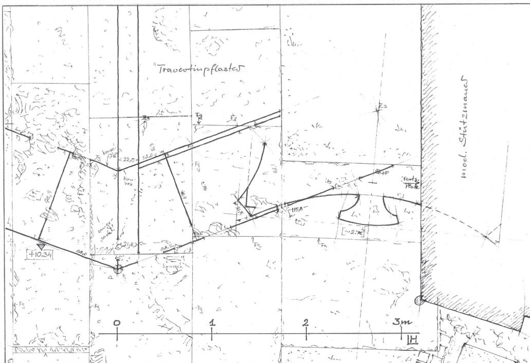
Fig. 5: Ancient construction drawings of the Mausoleum of Augustus, detail. Documentation plan with Corinthian pilaster capital and part of pediment (author).
