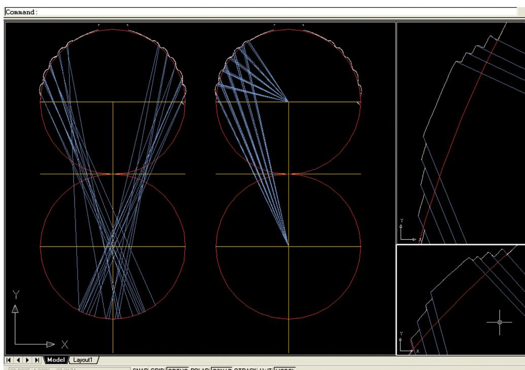
Fig. 10: Drawings examining the direction of the *lacunars*' section lines.
