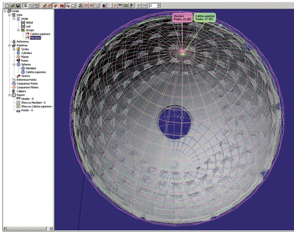
Fig. 5: The diameter of the *intrados*.
