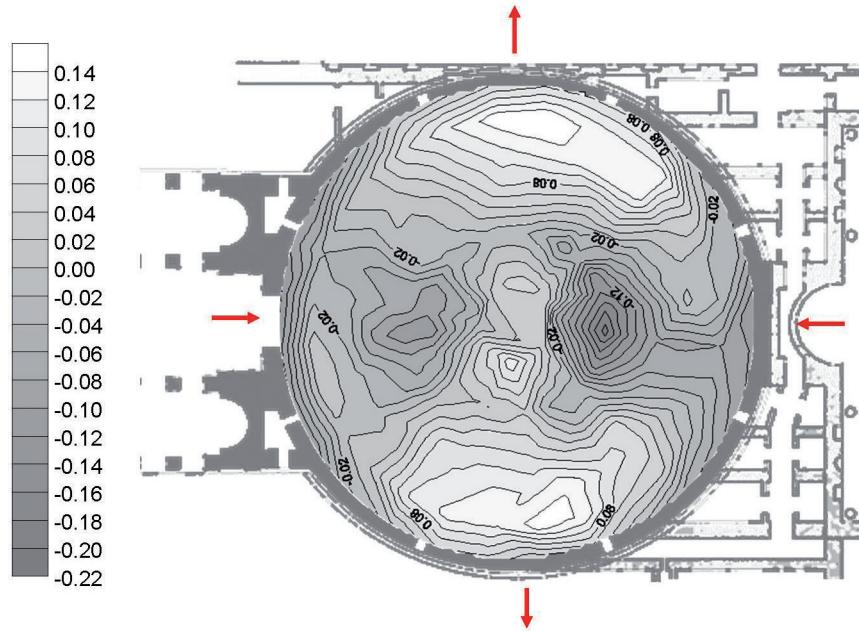
Fig. 8: Mid-distance-conform azimuthal mapping of the deviations of the dome.
