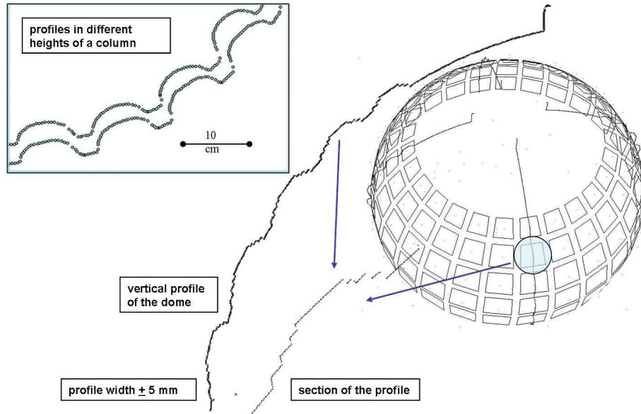
Fig. 6: Horizontal (left) and vertical profiles (right) of high precision.
