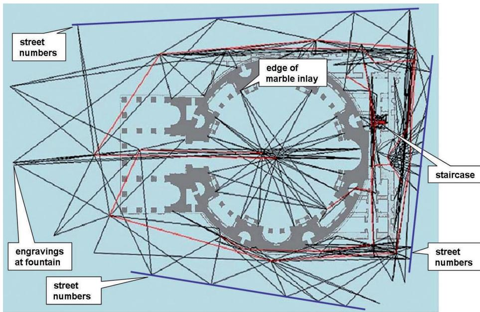
Fig. 2: Actual precise network of the Pantheon.
