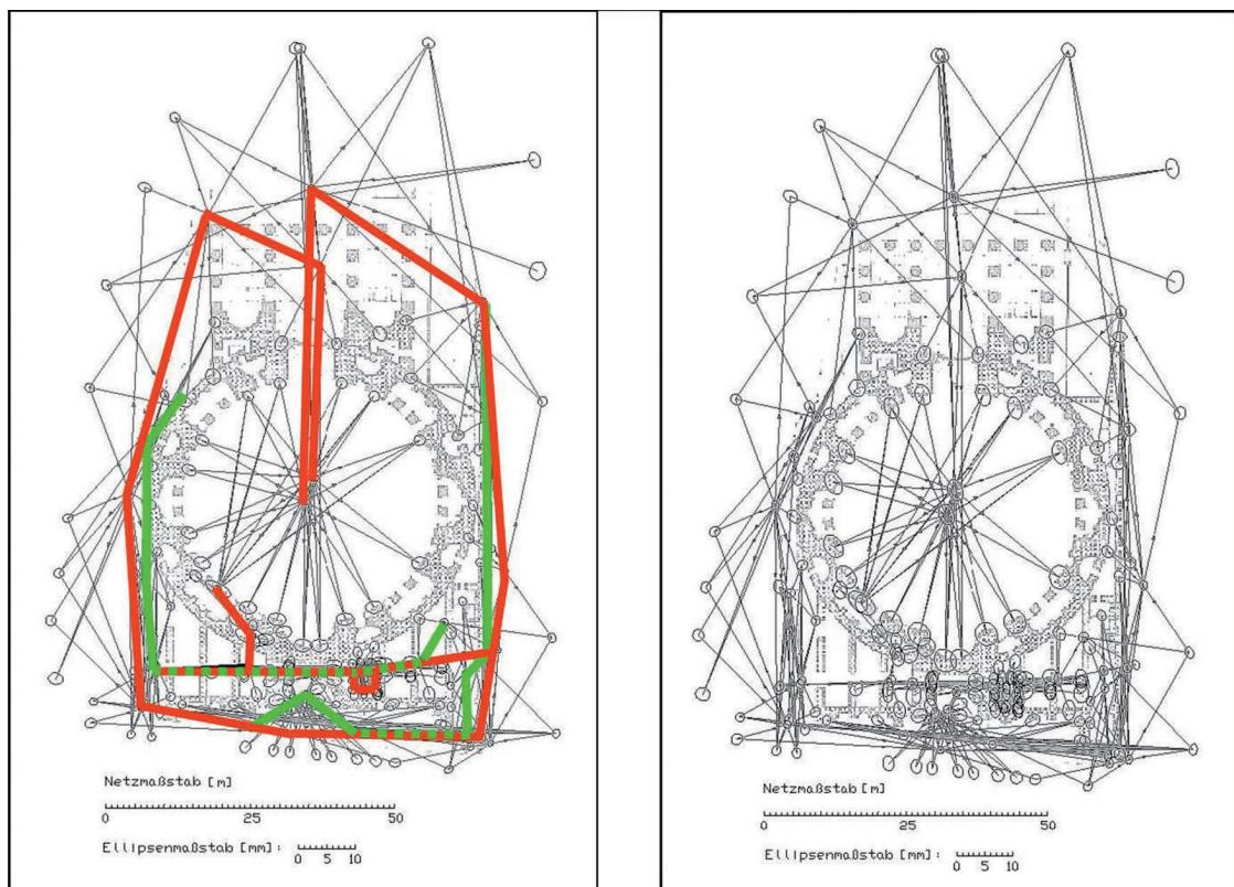
Fig. 3: Comparison of network accuracy obtained including the traverses (left) versus the accuracy obtained using micro-networks alone (right).
