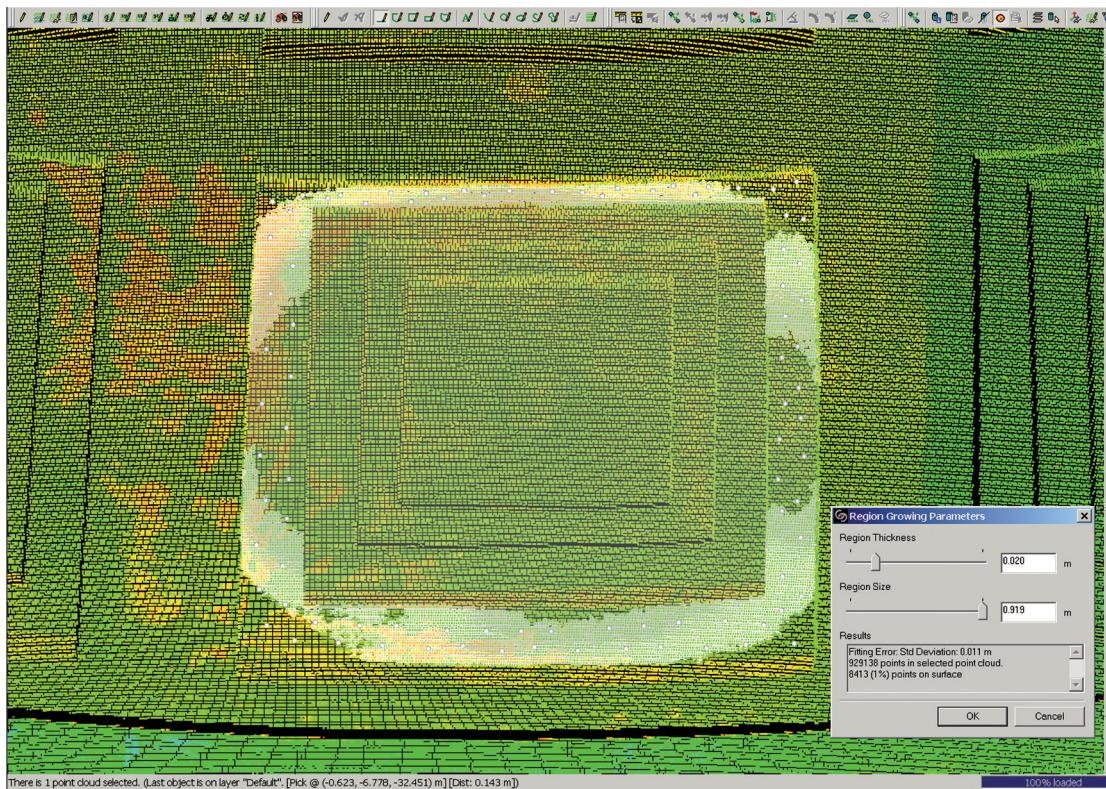
Fig. 6: The external surface of the *lacunars*, approximated by a plane (worse).
