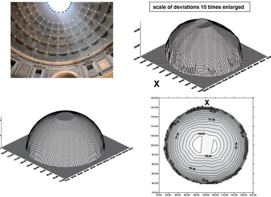
Fig. 7: Analysis of the spherical form of the dome.
