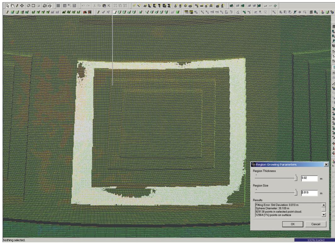
Fig. 7: The external surface of the lacunars, approximated by a sphere (better).
