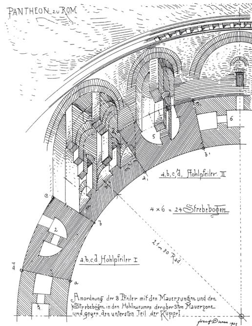
Fig. 3: Josef Durm, Pantheon: Perspective study of the drum’s third storey, 1903, from Durm 1905.
