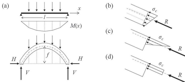
Fig. 4: Arch with thrust line; (a) beam analogy; (b) resulting force within core; resulting force outside core for (c) linear elastic and (d) perfect plastic material behaviour.
