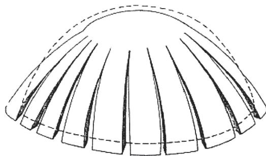
Fig. 2: Cracked cupola, according to Lucchini 1996.
