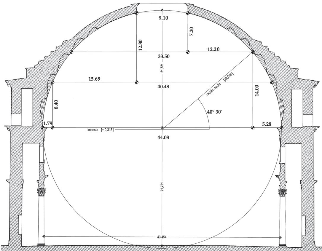
Fig. 6: Pantheon: Pelletti's measurements of the dome (1989), with additions by the author.
